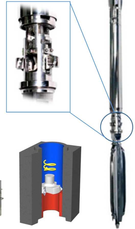
Graphite blocks calibration tool (horizontal cutting)
