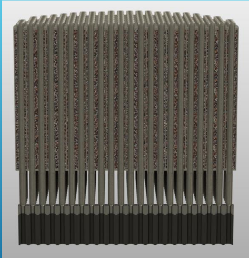
Figure 4. The upper pipe ends above the upper "E" scheme bars must be prepared and should be removed from the thermal cutting particles
